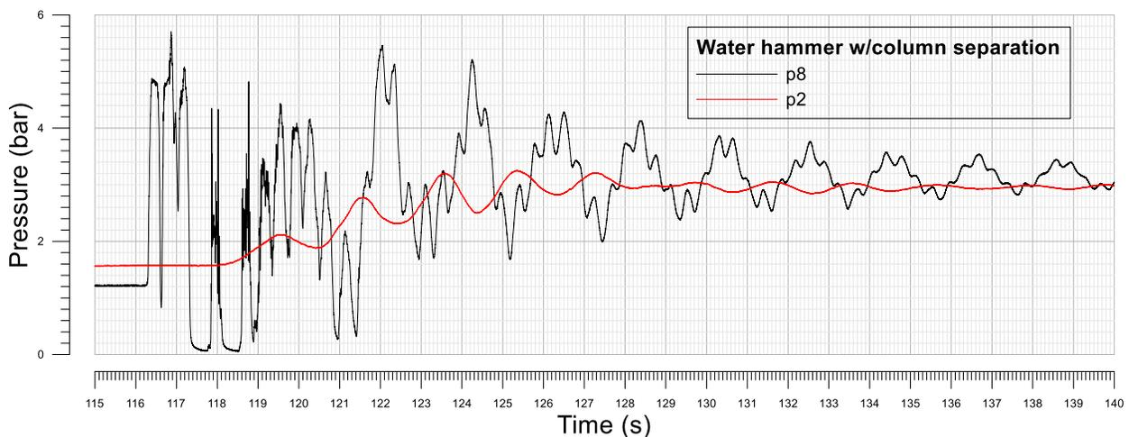
Time development of the measured pressure at two different locations separated more than 1000m apart and upstream of the closed valve. This result is from when air is still present in the system.
