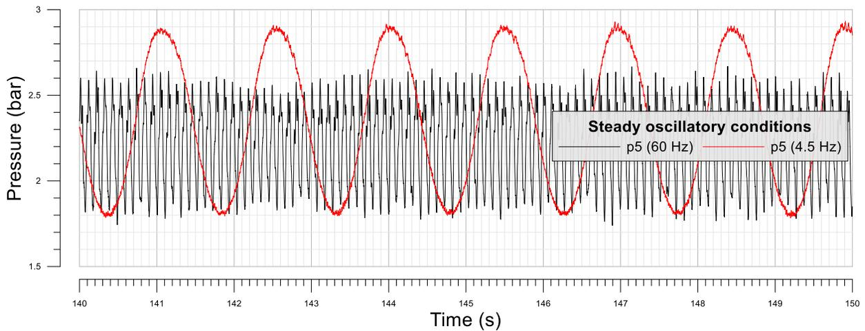
Pressure response from sensor roughly 600m upstream the oscillating valve for two driving frequencies. Note: Frequency indicated refers to motor driving frequency, and does not include gear transmission ratio.
