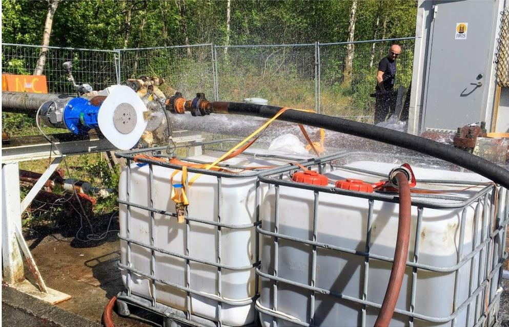
Picture of the valve for generating oscillatory flow in the system during operation. The white disc is connected to a motor shaft, operating at various frequencies. The disc rotates across a small slit in the outlet cross section, effectively changing the outlet area and the pressure loss across the valve. One can expect to get a little wet when this runs at full speed.
